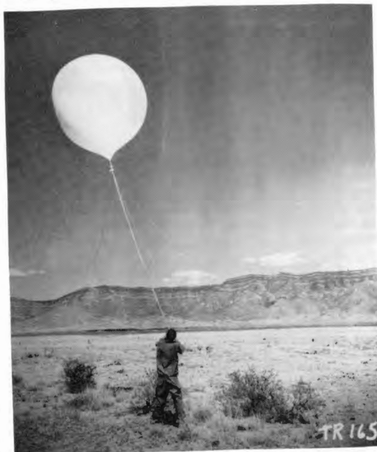
Figure 37. Helium balloon for raising primacord (TR-165).
