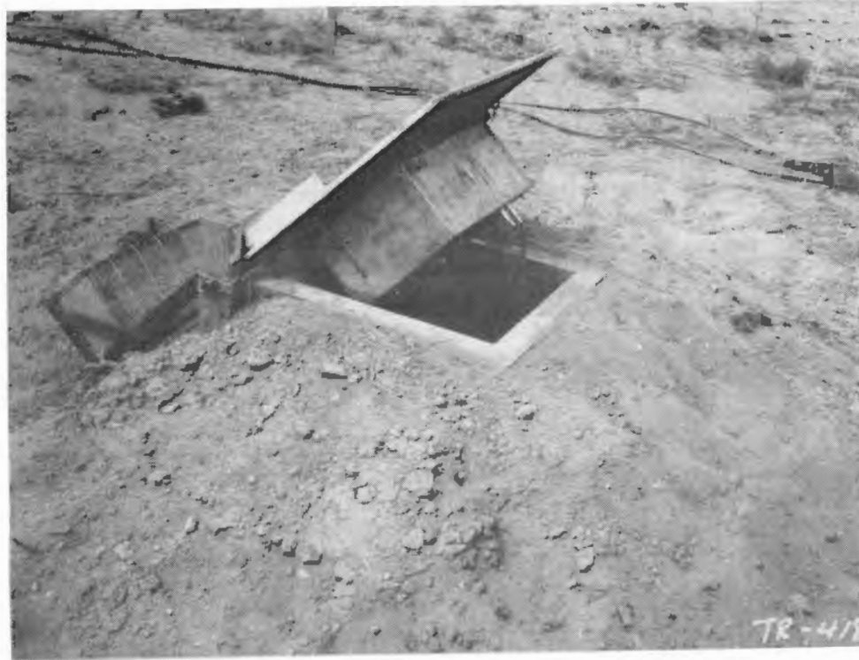
Figure 12. Type B gamma sentinel (TR-418).
