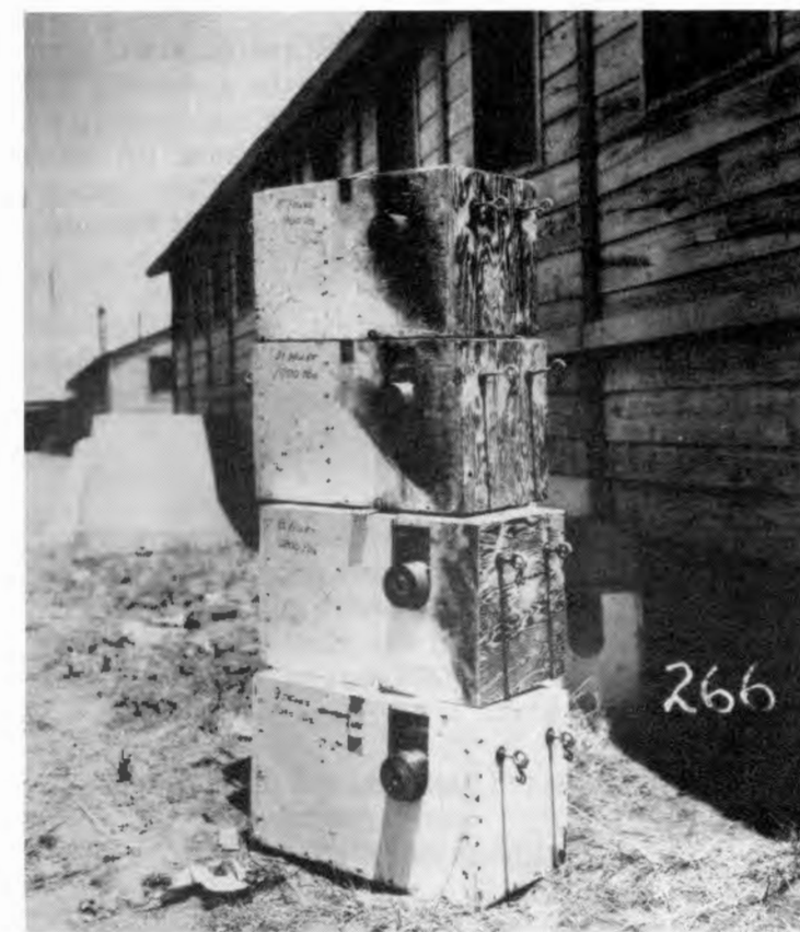
Figure 31. Impulse meters recovered after test (TR-266).
