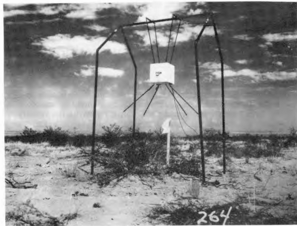
Figure 34. Excess velocity gauge before test (TR-264).
