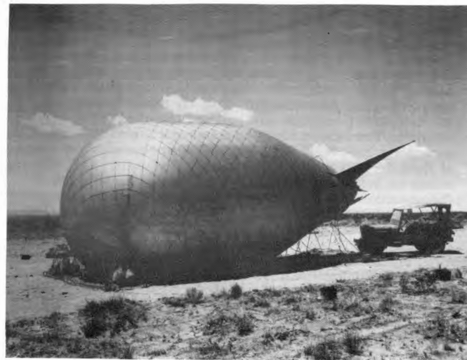
Figure 38. Barrage balloon for flying neutron camera (TR-393).
