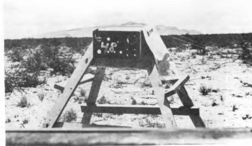
Figure 17. Paper box gauge after test (photo by J. Carlton Hoogterp).
