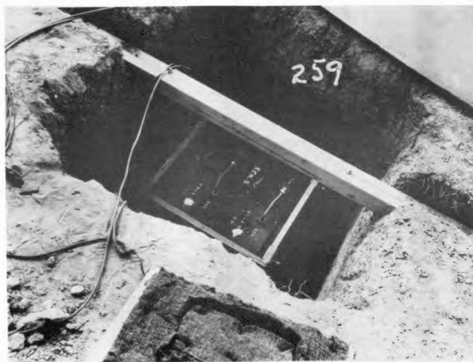
Figure 16. Geophone amplifiers after test (TR-259).
