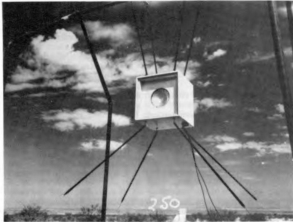
Figure 33. Excess velocity gauge before test (TR-250).
