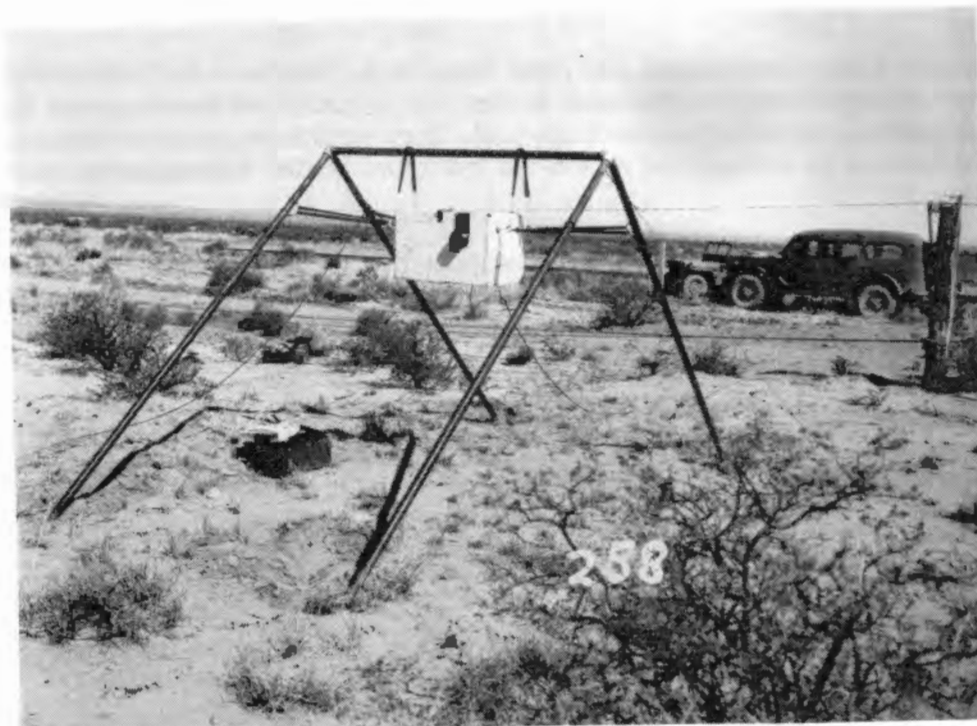
Figure 29. Impulse meter and stand before the test (TR-258).
