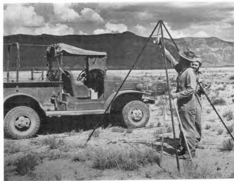
Figure 20. George A. Economou and Benjamin C. Benjamin (with hat) setting up Torpex charge tripod (TR-391A).
